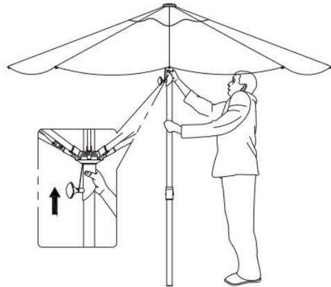
Push the handle upwards, as soon as the hole at the top is reached, you will hear a 'click' indicating that the screen is open and locked in place.
